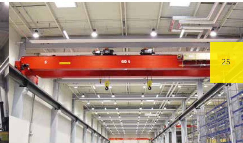
Double girder overhead travelling bridge crane
