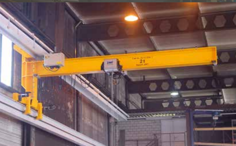
Wall console crane
