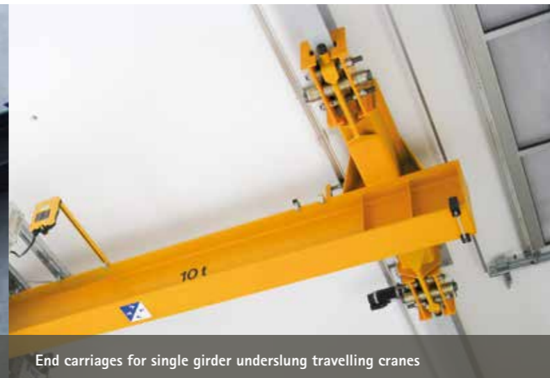
End carriages for underslung cranes with standard connection and painting as an option
