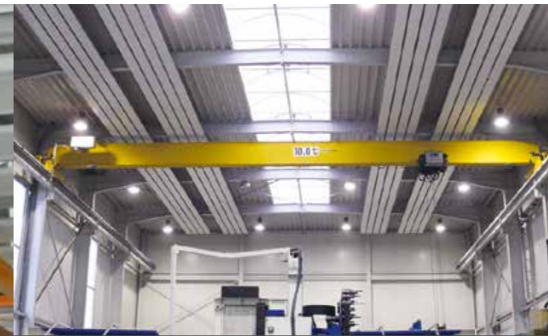
Single girder overhead travelling bridge crane
