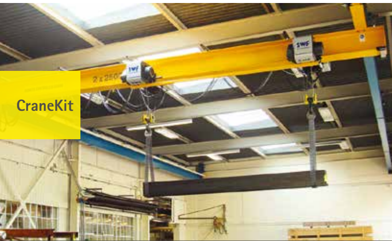
Single girder underslung travelling crane
