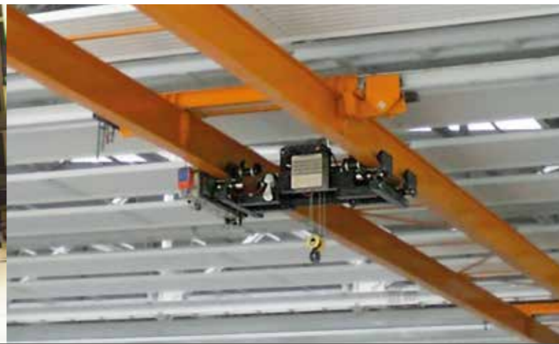
Double girder underslung travelling crane
